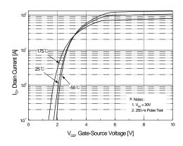
Figure 2. Transfer Characteristics
