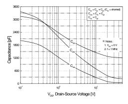
Figure 5. Capacitance Characteristics
